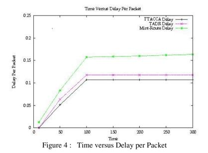
(iii) Delay: The time taken between the source node sending the packet and the destination node receiving the packet is End-to-End Delay.
