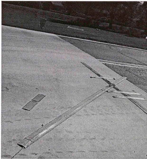
Figure 5-9 On-campus test site for single element vehicle classification system
