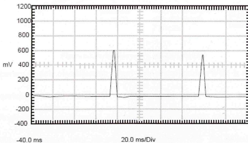
Figure 2-2 Pulses produced by axles hitting a piezoelectric sensor [22]
