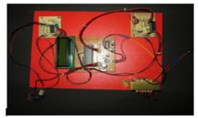
Figure 9: Snapshot of the Transmitter Section
