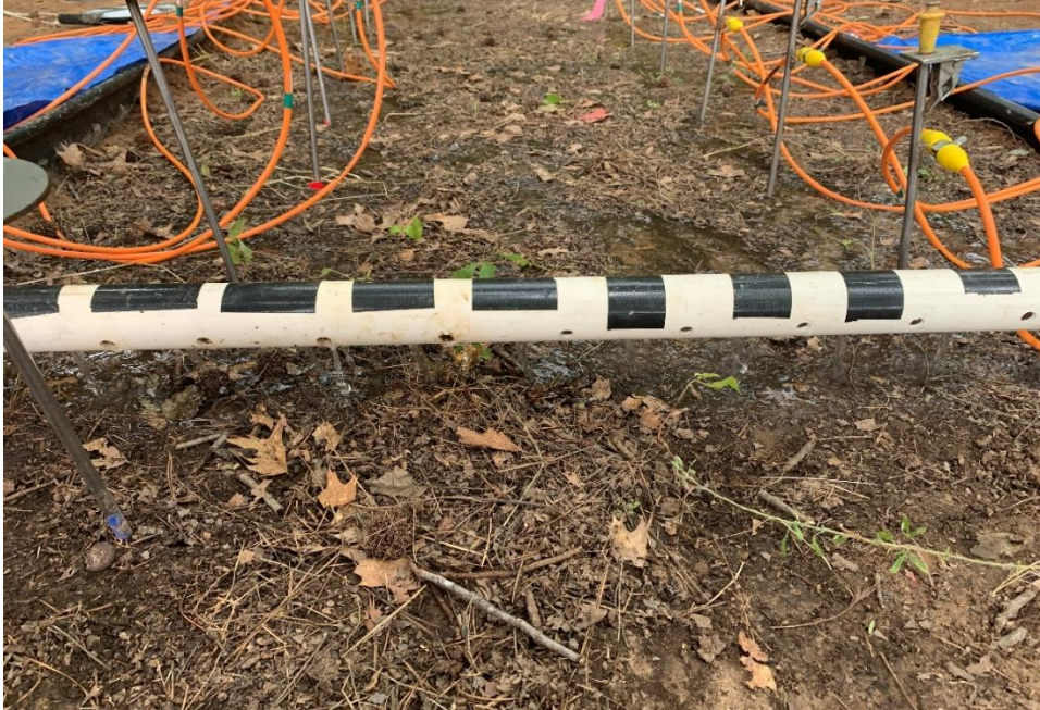
Figure 10 - Field photo of the wetting source for the wetting domain in North Carolina.
