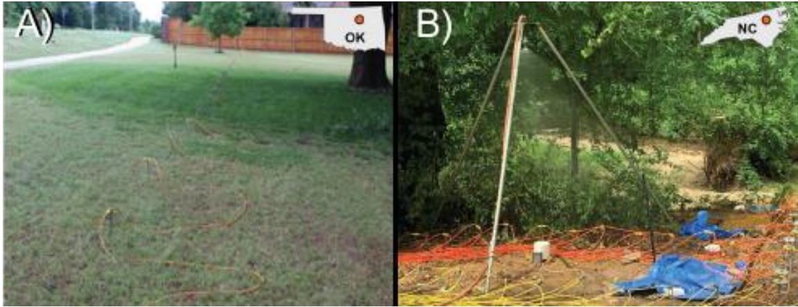
Figure 1 - Field sites for TERI experiments. A) ERI line in fine grain soil site in Oklahoma. Orange cable connects 28 stainless steel electrodes at a 1.6 meter spacing in fine soil. B) ERI line in coarse grain soil site in North Carolina. The orange cable connected the electrodes in the ground to the resistivity instrument utilized for this work. The white cylinder below the sprinkler tripod is the rain gauge used for measuring precipitation. 28 electrodes at 0.4 meters spacing were utilized for the experiment.
