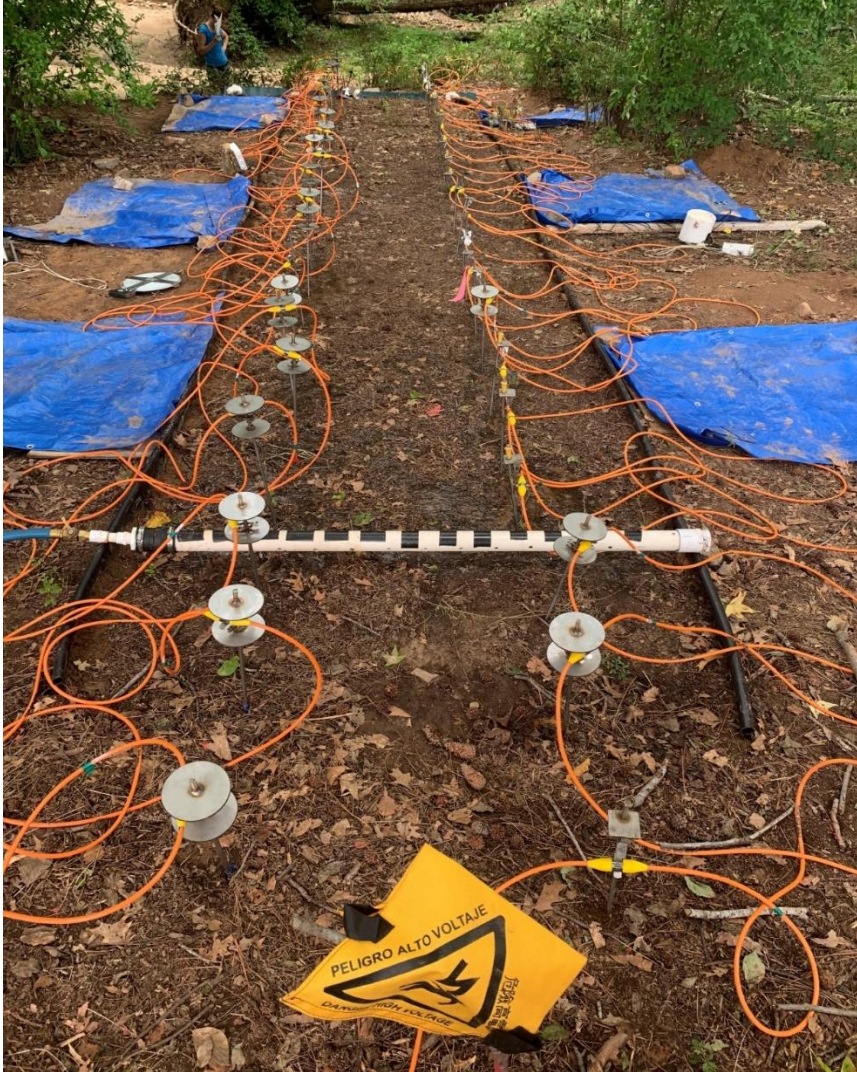
Figure 9 - Field photo of the entire wetting domain in the North Carolina site. Line 1 is on the left, line 2 is on the right. The wetting source is the black and white pvc pipe in the foreground, Soil pits are covered in blue tarps.
