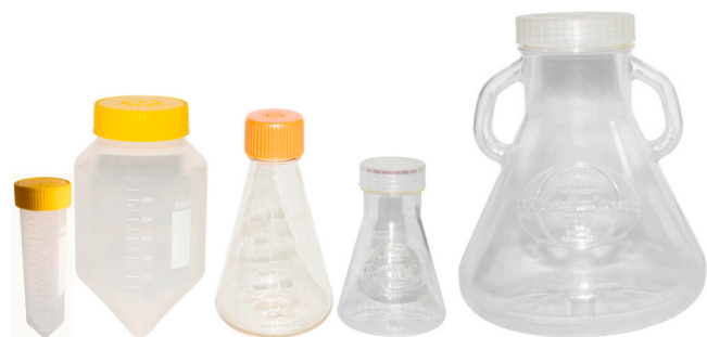
Fig. 2. Depiction of the investigated disposable orbitally shaken cultivation systems. From left to right: 50 and 600 mL TubeSpin (made of polypropylene), 500 mL Erlenmeyer flask (made of polycarbonate), 500 and 5000 mL Optimum Growth flask (made of polypropylene).
