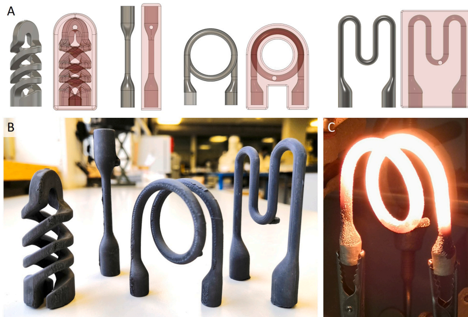
Fig. 4. Examples of heating elements designed for injection molding using 3D printed PVA molds. CAD drawings of the target parts together with the respective PVA molds (A). Green bodies after injection molding and dissolving the PVA molds (B). Sintered spiral part in glowing test at 460 W power input (C).
