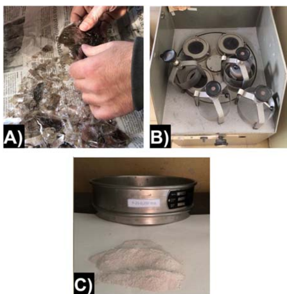
Figure 2. Manual breaking (a), milling (b) and sieving (c) process of mica mineral.
