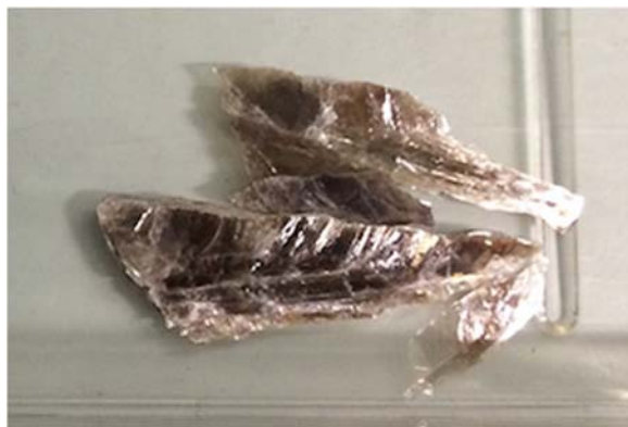
Figure 1. Mica mineral pieces used for electron microprobe analysis.
