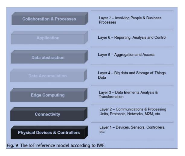
Figure 5- The IoT reference model according to IWF.
