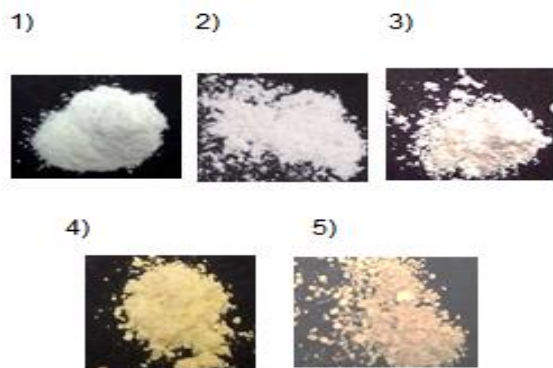
Imagen 1. Color desarrollado por los pigmentos: 1) \text{Eu}_{0.93}\text{Gd}_{0.07}\text{AlO}_3 , 2) \text{Eu}_{0.93}\text{Dy}_{0.07}\text{AlO}_3 , 3) \text{Eu}_{0.93}\text{Er}_{0.07}\text{AlO}_3 , 4) \text{Eu}_{0.93}\text{Pr}_{0.07}\text{AlO}_3 , 5) \text{PrAl}_{0.93}\text{Cr}_{0.07}\text{O}_3 .
