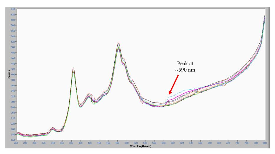
Figure 22. MSP Emission Spectra of Polyester Fibers (Two Discriminated by FL 546 Filter), FL 546, 40x objective.
