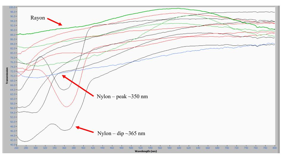
Figure 18. MSP Spectra of All Non-Polyester Fiber Samples, 10x objective.
