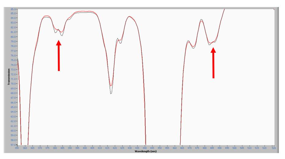
Figure 9. MSP Spectra of Holmium Oxide Filter, Resolution Factor Study (1 vs. 2), 40x objective.
