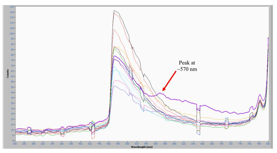
Figure 21. MSP Emission Spectra of Polyester Fibers (One Completely Discriminated by FL 420 Filter), FL 420, 40x objective.
