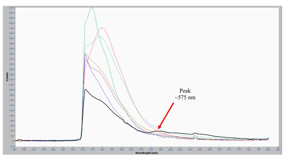
**Figure 20.** MSP Emission Spectra Representative of Seven Groups of Polyester Fibers (No Additional Peaks in Transmission) Separated by the FL 365 Filter, FL 365, 40x objective.
