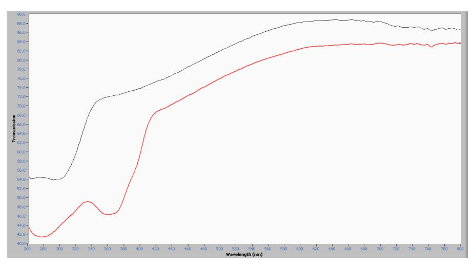
Figure 25. MSP Spectra of Physically & Optically Similar Fibers from Figure 24, 10x objective.
