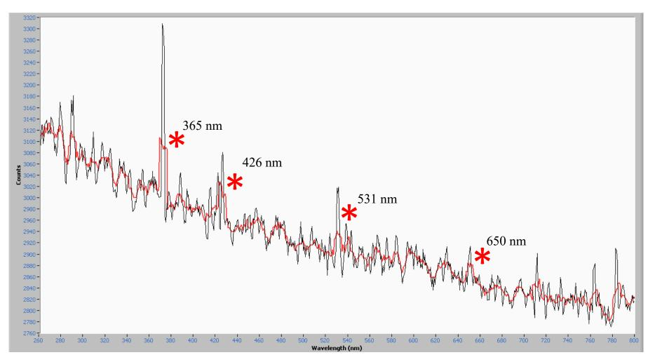
Figure 11. MSP Emission Spectra of Fluorescence Dark Scans, Resolution Factor Study (Fluorescence), 40x objective.
