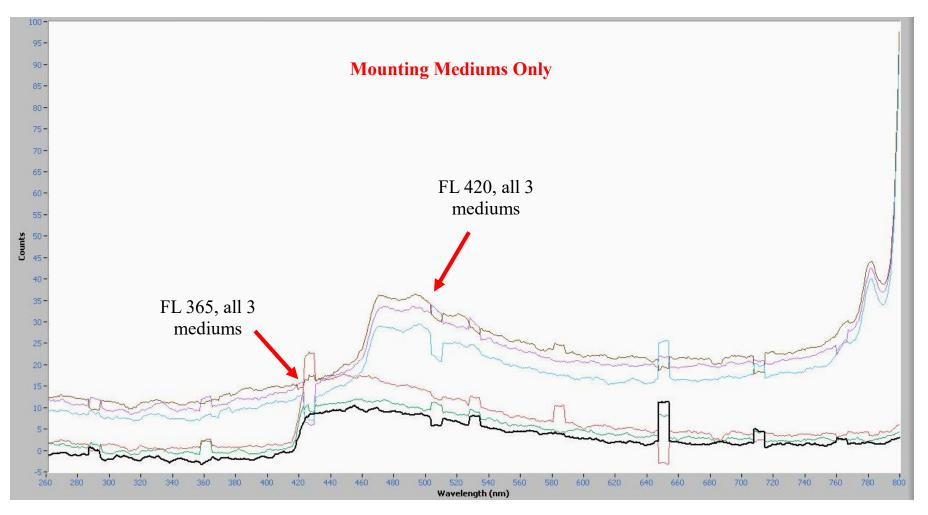
Figure 14. MSP Emission Spectra of Mounting Mediums (FL 365 & 420), Mounting Medium Study, 40x objective.
