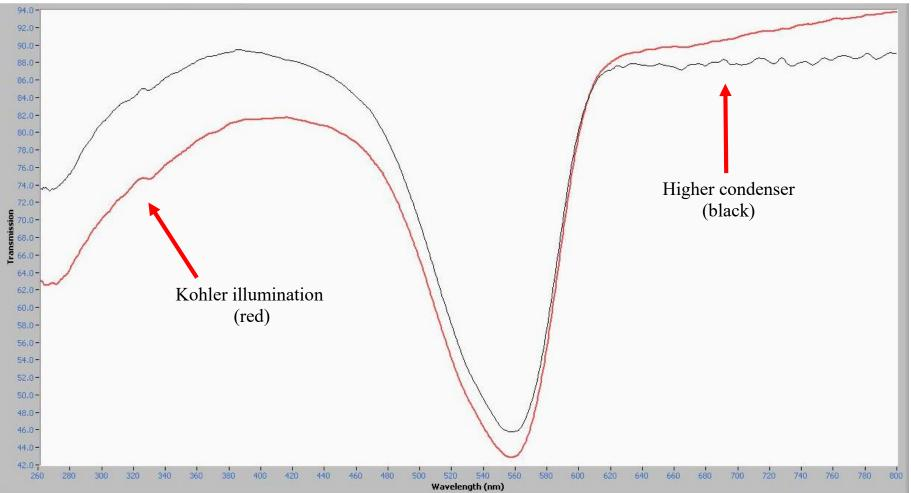
Figure 3. MSP Spectra of Neon Pink Acrylic Fiber, Condenser Study, 10x objective.
