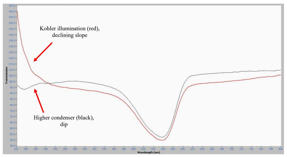
Figure 4. MSP Spectra of Neon Pink Acrylic Fiber, Condenser Study, 40x objective.
