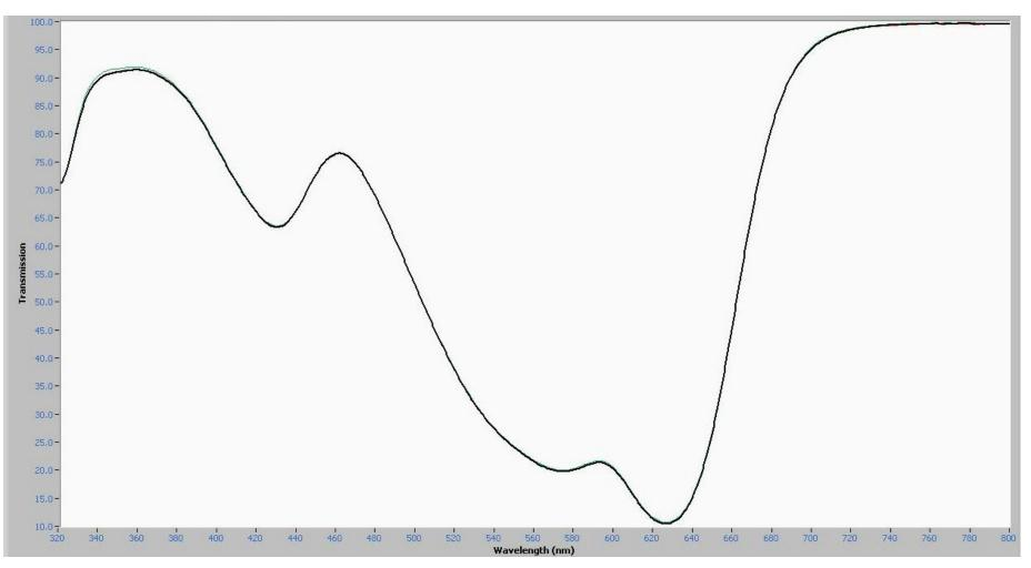
Figure 7. MSP Spectra of Dark Blue Acrylic Fiber, Number of Scans Study, 10x objective.
