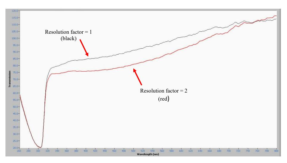
Figure 10. MSP Spectra of #150 Polyester Fiber (Colorless), Resolution Factor Study (1 vs. 2), 40x objective.
