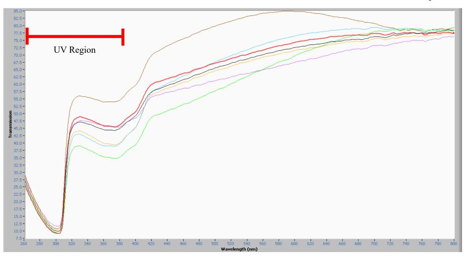
Figure 17. MSP Spectra of One Group of Polyester Fiber Samples, 10x objective.
