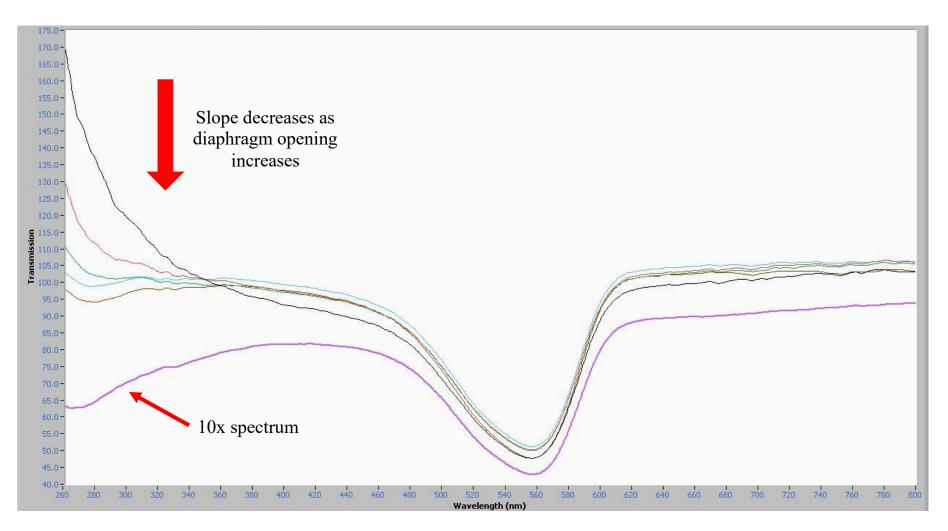
Figure 5. MSP Spectra of Neon Pink Acrylic Fiber, Field Diaphragm Adjustments, 40x objective.
