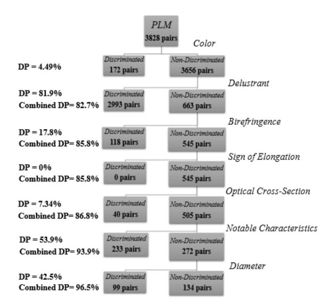
Figure 23. Discrimination Power of Colorless Fibers by PLM.
