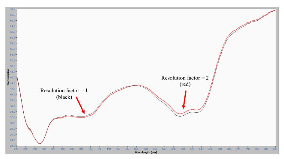
Figure 8. MSP Spectra of F516 Polyester Fiber (Blue), Resolution Factor Study (1 vs. 2), 10x objective.
