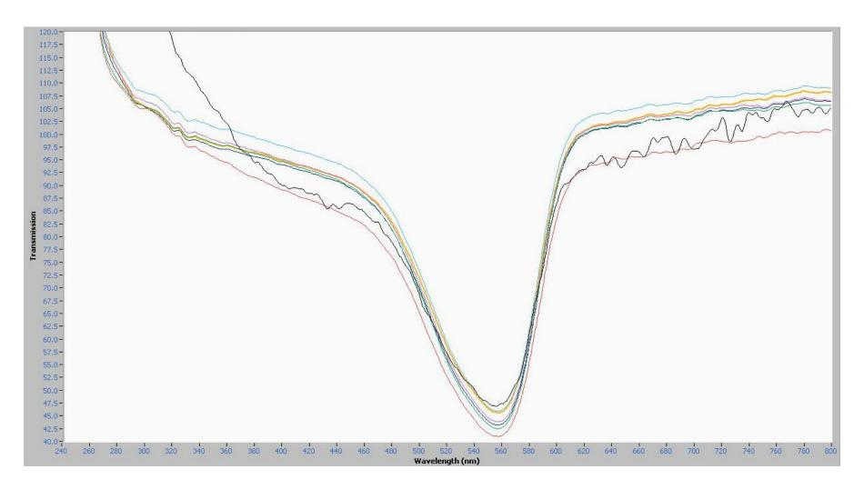
Figure 6. MSP Spectra of Neon Pink Acrylic Fiber, Iris Opening Study, 40x objective.
