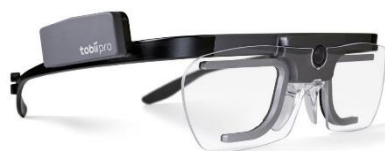
Εικόνα 3 Wearable eye tracker ( https://www.tobii.com/imagevault/publishedmedia/8clvxud7x9j3fqte76kj/TobiiPro_Glasses_2_Eye_Tracker_side_2_1.jpg )
