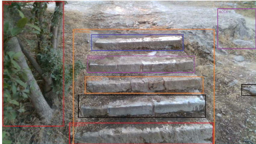
Figure 6.6 Classification example of 8 obstacle regions using the proposed architecture with 5 workers. Each color corresponds to a different worker.
