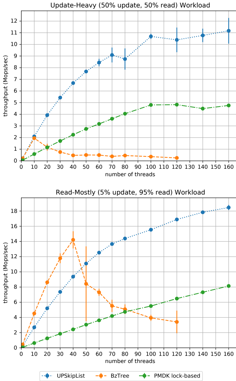
Figure 5.1: Throughput comparison using YCSB benchmark workloads A and B for UP-SkipList, BzTree, and the PMDK lock-based skip list.
