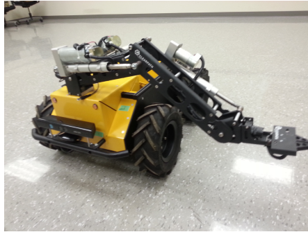
Fig. 5 Clearpath manipulator mounted on a Clearpath A200 mobile platform.
