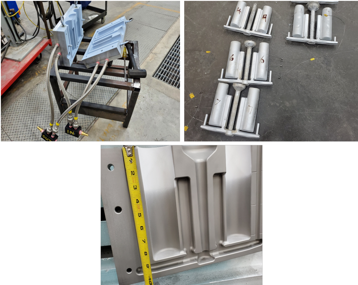
Figure A.2: Detailed images of the cylinder casting mould, showing water cooling lines, detailed mould geometry and approximate size, and the casting. Images courtesy of Peter Newcombe at CANMETMaterials.
