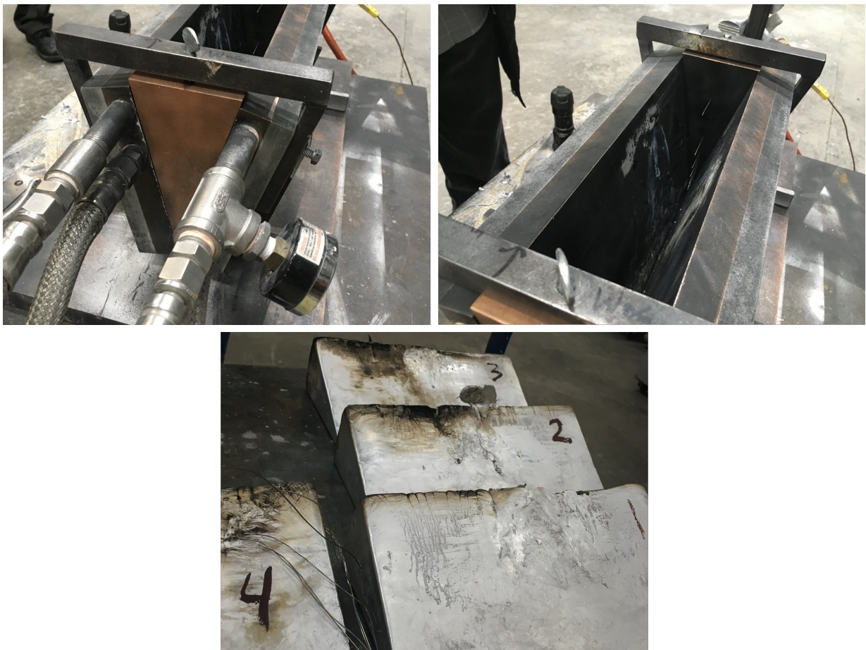
Figure A.1: Detailed images of the wedge casting mould, showing water cooling lines, thermocouples inside the mould, and the cast wedges.
