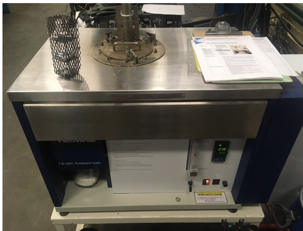
Figure 4.6: The fluidized alumina powder bath, and wire-mesh cage, used for homogenization treatment.
