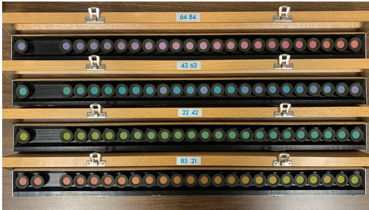
Figure 1.3: The Farnsworth Munsell 100 Hue test. From bottom to top, tray 1 is nominally red to red-orange, 2 is yellow to yellow-green, 3 is green to green-blue and 4 is indigo to indigo-magenta.
