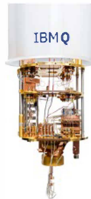
Figure 1: IBM's 50 qubit quantum computer
