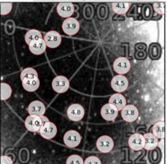
By obtaining a FITS image by the AllSky 340 Camera, we used an astrometric calibration service website known as astrometry.net. where we uploaded it to. This website delivers information not just where each star is positioned, but as well as their photo-electron count, in other words, the amount of photons the camera received in a given image.
