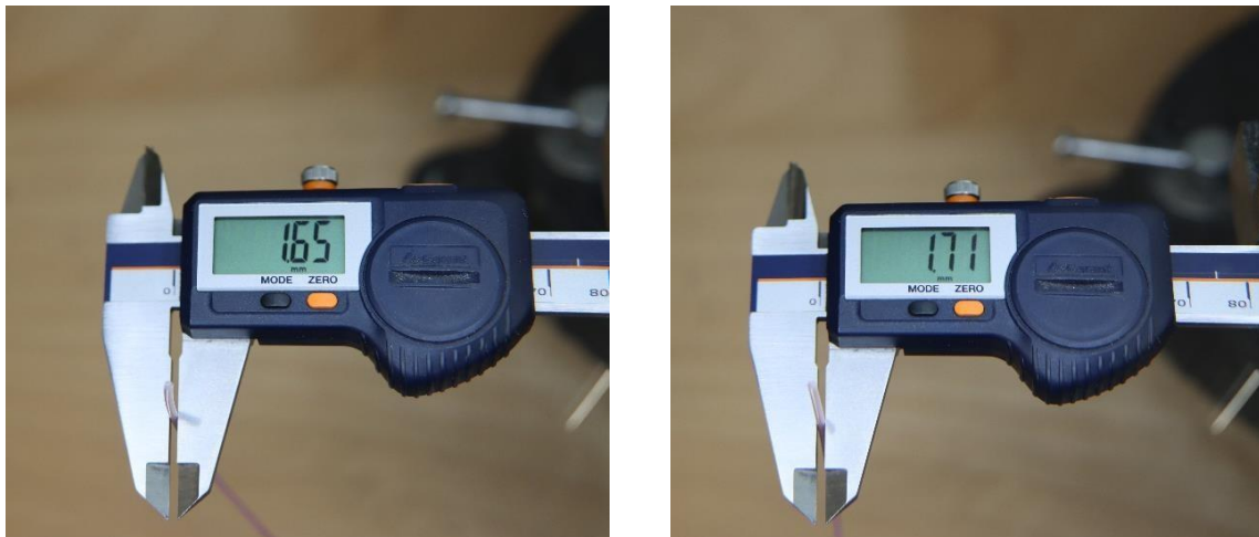
Figure 3.10 – Measurement of the dimensional filament control, (left – D1), (right – D2).
