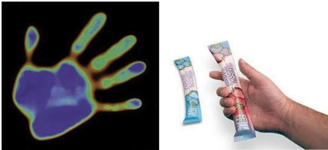
Figure 2.10 – Thermochromic liquid crystal ink representation [56] (left), colour change – Printing package (right)[57].
