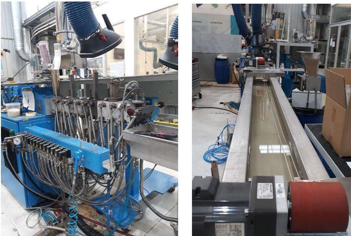
Figure 3.5 – Extrusion machine (left), cooling zone (right).
