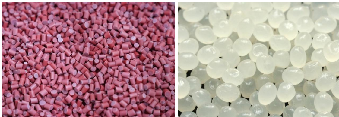
Figure 3.1 – Granular thermochromic masterbatch (left), granular polymeric matrix of PLA (right).
