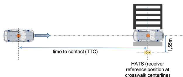
Fig. 6. Time between a moving object on a collision path to an observer may be defined by a relation between its distance and velocity. Frequently, the terms time-to-contact (TTC), time-to-arrival (TTA) or time-to-collision (ITC), are employed for this measure. Schematic representation in the context of the current study.
