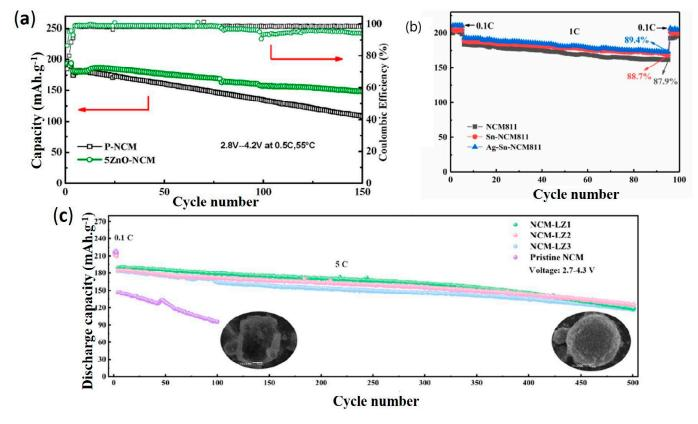
**Figure 6.** (a) Cyclic performance at 55 °C of NCM and 5ZnO-NCM [150], (b) Cycling performance of NCM811, Sn-NCM811, and Ag-Sn-NCM811 (1 C =  $200 \text{ mA} \cdot \text{g}^{-1}$ , at the range of 2.8–4.3 V) [151], and (c) Cycling performance of the a La<sub>2</sub>Zr<sub>2</sub>O<sub>7</sub>-coated NCM samples at 5 C [153].
