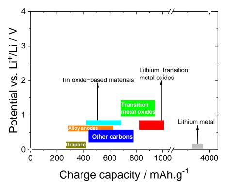
**Figure 2.** Voltage range vs. Li/Li<sup>+</sup> as a function of the charge capacity of different anode active materials (adapted from [61]) [59].
