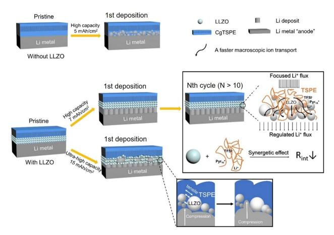
Figure 9. Effect of an LLZO layer in the suppression of lithium dendrites growth [29].
