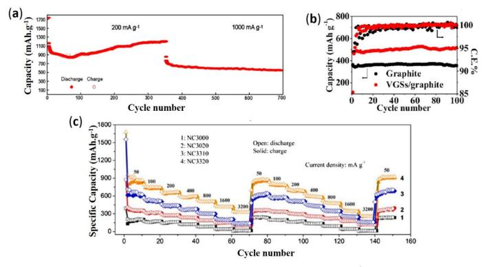
**Figure 3.** (a) Long-term cycling performance of  $CoCl_2$ -Fe $Cl_3$ -GICs at 200 and 1000 mA·g<sup>-1</sup> [66]. (b) Cycling curves of graphite and vertical graphene sheets (VGSs)/graphite at 0.2 C [67]. (c) Rate performance at various current densities for the different nitrogen-doped graphene-like carbon nanosheets samples [68].
