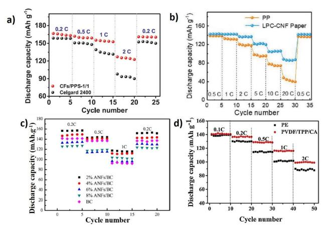
**Figure 8.** (a) Discharge C-rate capabilities of cells with Celgard 2400 separator and CFs/PPS-1/1 separator [212], (b) Rate capability of LFP half cells with PP and LPC-CNF paper separators at different current densities [231], (c) Rate capability of LFP half-cells with BC and ANFs/BC separators [200], and (d) Rate capabilities of LFP half cells using PE and PVDF/TPP/CA membranes [237].
