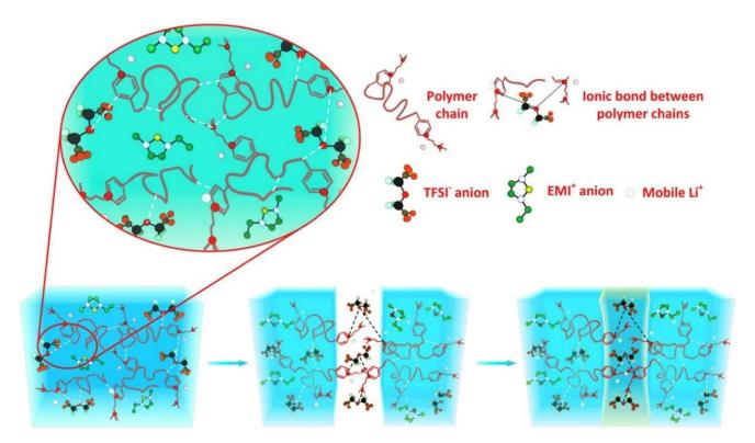
Figure 10. Self-healing mechanism in a PIL-based SPE [261].
