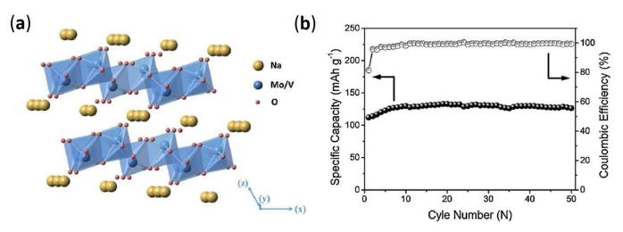
Figure 7. (a) Schematic structure and (b) battery performance for NaVMoO<sub>6</sub> [179].
