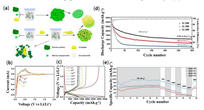
**Figure 4.** (a) Schematic illustration of the preparation process of amorphous carbon-coated silicon [74], (b) CV curves of Si-200 at a scan rate of 0.1 mV·s<sup>-1</sup>; (c) Galvanostatic discharge/charge profiles of Si-200 at 0.2 A·g<sup>-1</sup>; (d) Cycling performance of various nano-Si at 0.2 A·g<sup>-1</sup> [81]; and (e) Rate capability of the different silicon oxycarbide (SiOC) samples measured at various C-rates from 180 to 3600 mA·g<sup>-1</sup> [82].
