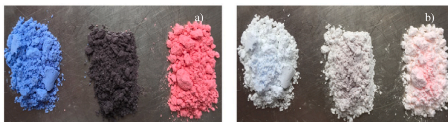
Fig. 9. Thermochromic powders (blue, black, and red): a) deactivated below 31 °C and b) activated above 31 °C (right) [113].
