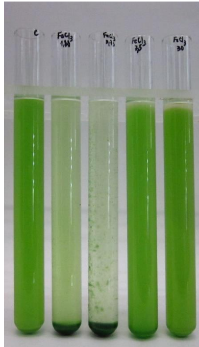
Figure 3.14 Comparison of the results of M. aeruginosa harvesting using four different \text{FeCl}_3 concentrations after 2 hours of treatment: control; 1.88 \text{ mg.L}^{-1} ; 3.75 \text{ mg.L}^{-1} ; 7.5 \text{ mg.L}^{-1} , and 15 \text{ mg.L}^{-1} .
