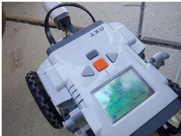
Figure 1. The NXT Smart Brick of the Mindstorms NXT 2.0 LEGO robotics kits
