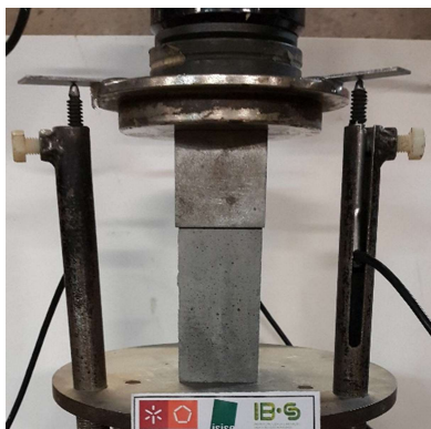
Figure 3. Test setup of compressive test
