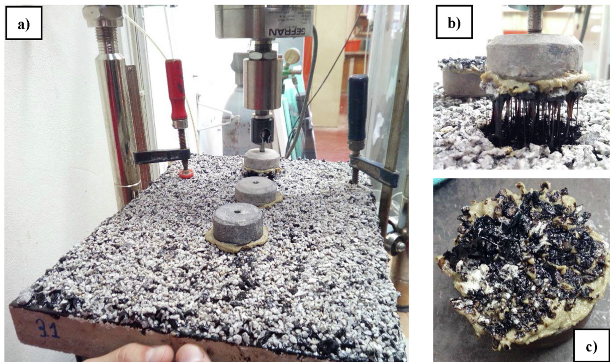
Fig. 4. Pull-off test: a) position of the plates; b) removal of the surface dressing; c) final aspect of the removed surface dressing.
