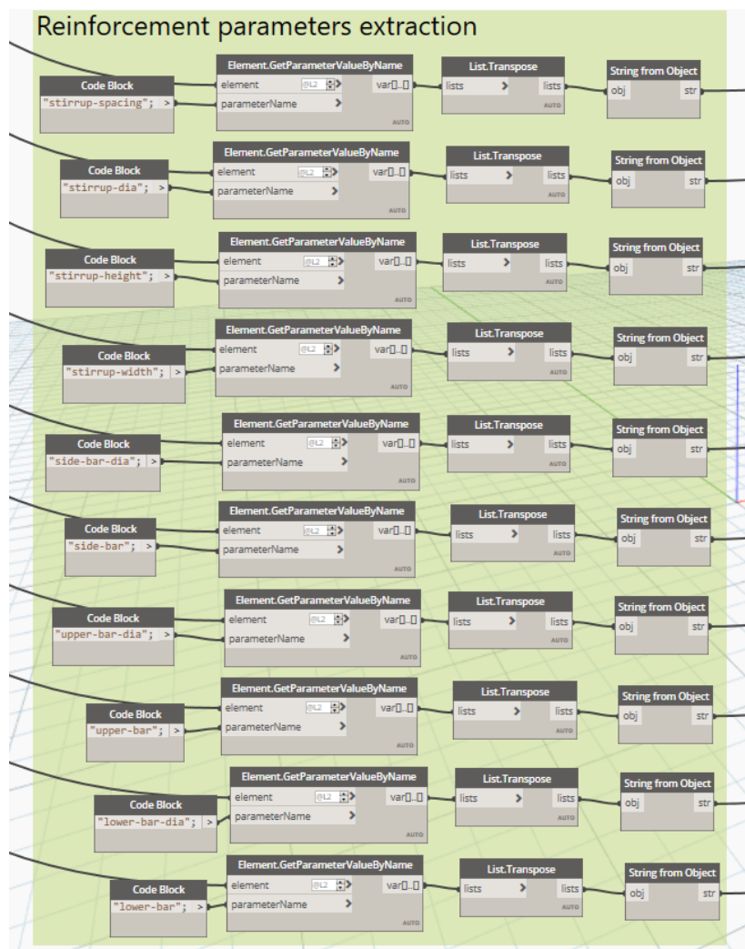
Figure 1-3 Extraction of reinforcement parameters
