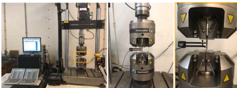
Fig. 3. Mechanical testing system used to perform the tensile tests.
