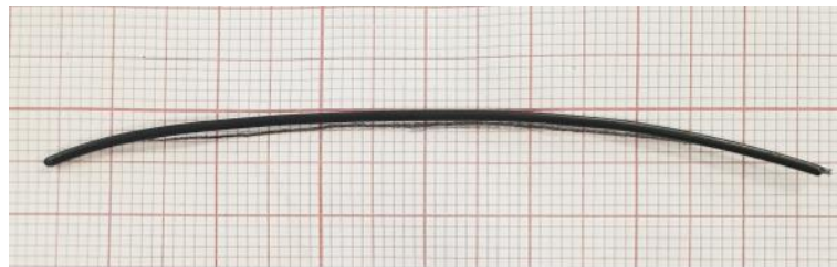
Figure 7-6: Shape of the nitinol wire after heating above A_f - austenite shape.
