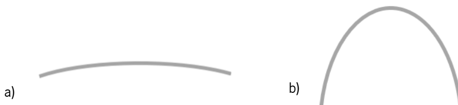
Figure 7-9: Representation of the expected final shapes of the nitinol wire in a) austenite phase and b) martensite phase.
