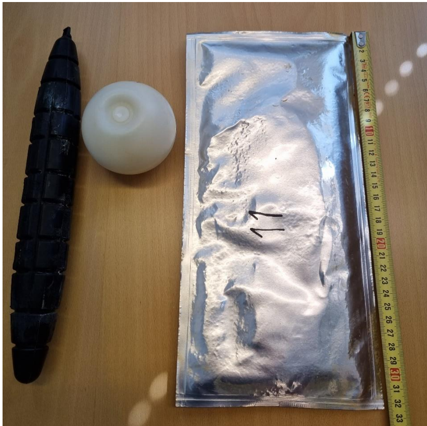
Figure 21 Acquired materials for testing with measurement tape for scale. Materials from left to right: Axiotherm HeatStixx capsule (ATS58 and ATP60), Global-E-System B.V. Gaia HS PCM58, and Climator AB ClimSel C58.
