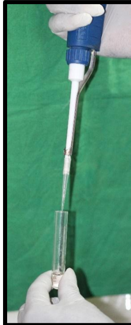
23 (A): Addition of sodium azide solution to the glucose reagent
