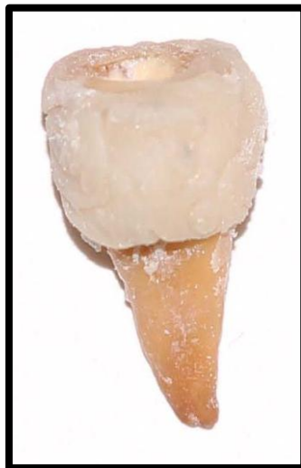
Figure 21: Cylindrical self cure acrylic arround specimen
