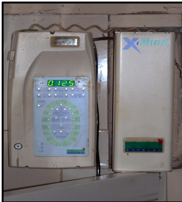
Figure 2: Satelec X- ray unit (70kVp, 8mA) Class 1 type
