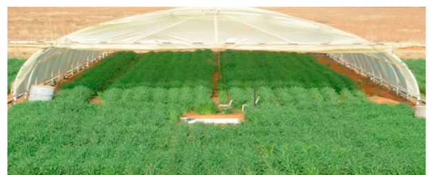
Figure 3. Wheat under the movable shelter (30 m long, 10 m wide and 4 m high), covering the lysimeter unit to prevent the influence of rain.
