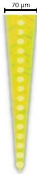
Figure 2. Image of a Michigan microelectrode system, or Michigan probe, with lithographically-modified recording sites on the surface of the silicon planar shank (21) .
