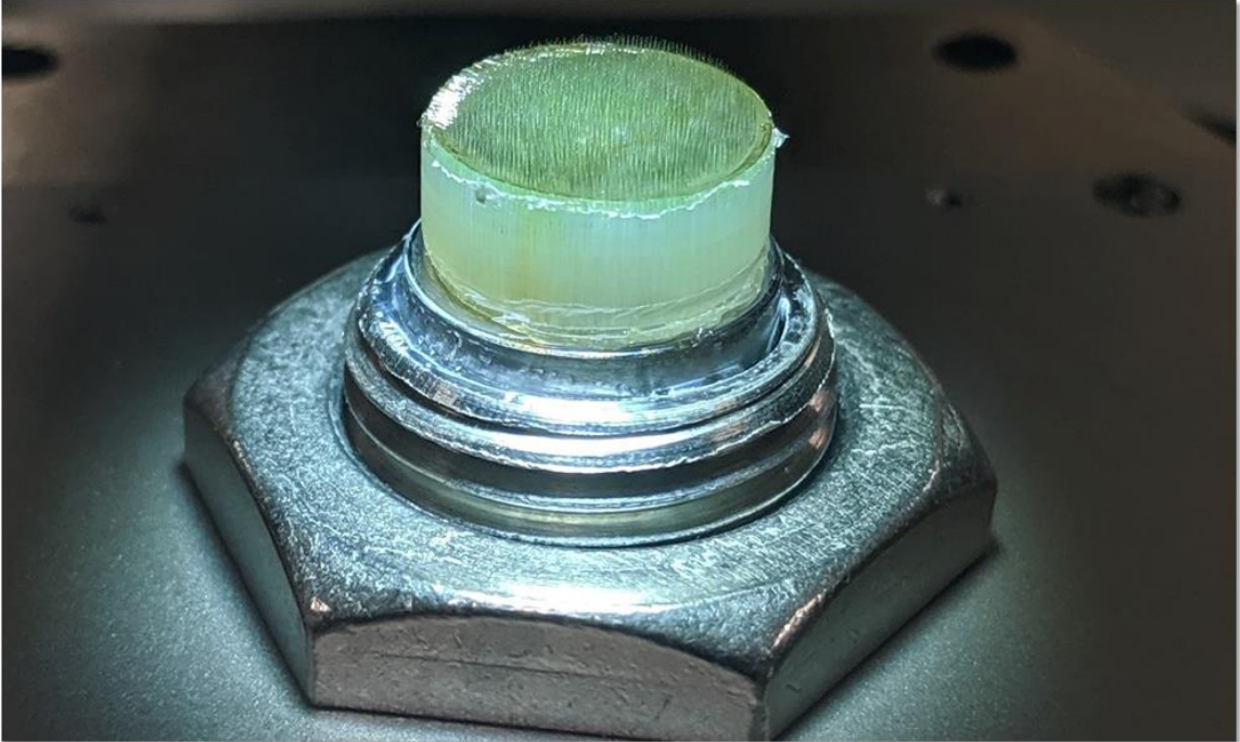
Figure 9. A fully fabricated microwire electrode array threaded onto the front plate (32) .
