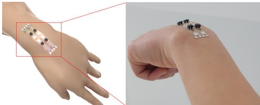
Figure 2.44. Schematic illustration and photograph showing the flexible/stretchable Ag 2 S-based RRAM system.
