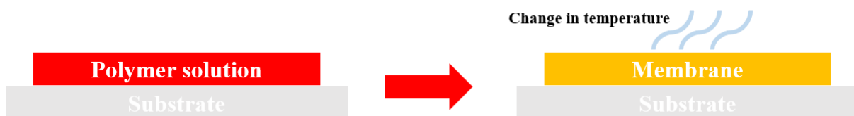
Figure 2. 2 Membrane fabrication caused by temperature difference in TIPS process.
