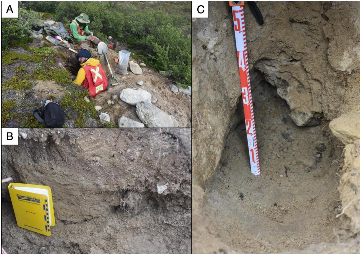
Figure 2.8: Glaciofluvial hummock sampling and grain size investigation. A) Sampling site. B) Glaciofluvial hummock displaying weakly stratified sandy nature of the sediment. C) Glaciofluvial hummock displaying the sandy diamicton with in situ boulders and cobbles.
