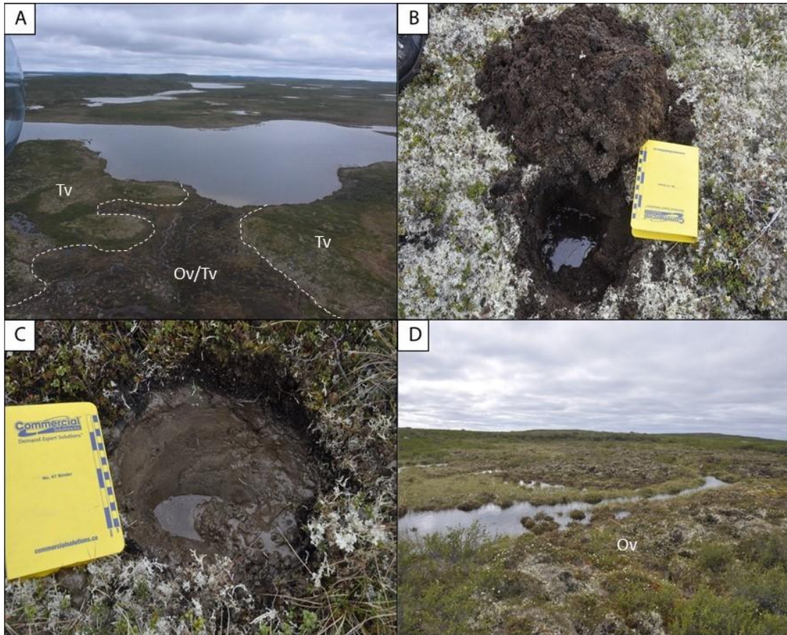
Figure 2.4: Organic materials A) Aerial view of organic veneer proximal to a lake. B) A pit in organic deposit; groundwater is commonly encountered. C) A pit with organics overlying silty sediments and groundwater table near surface. D) A wetland area containing tuffs of organics.
