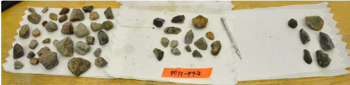
Figure 3.6: An example of a pebble lithology sample (PD19-P47) that has been sorted into the three broad lithology groups. From left to right: granitoids, meta-volcanics and meta-sedimentary.
