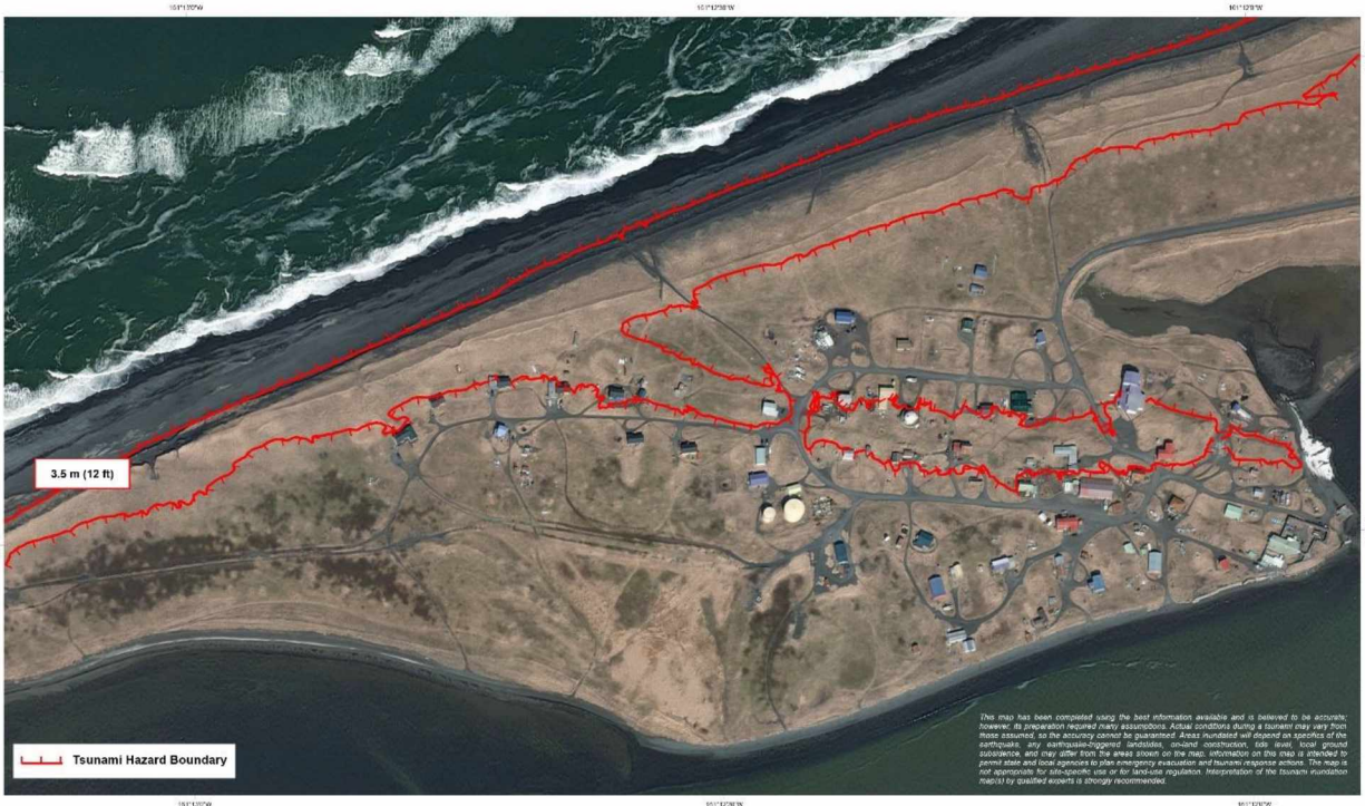
Figure 38. Tsunami hazard map of Nelson Lagoon, produced by the Alaska Earthquake Center for the Alaska Department of Geologic and Geophysical Surveys (from Suleimani et al., 2020). Information on this map is intended to permit state and local agencies to plan emergency evacuation and tsunami response actions. The map is not appropriate for site-specific use or for land-use regulation. Notice that the spatial pattern of vulnerability matches that of the SVTM produced by this project (see figure 32).
