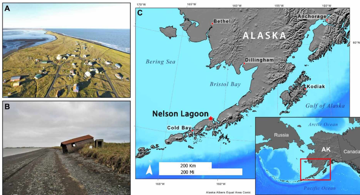
Figure 1. Study site map of the Native Village of Nelson Lagoon. (A) UAV imagery over the residential portion of the community. The right side of the image is the Bering Sea, left side is the back-barrier lagoon. (B) Cross-shore image showing set-net cabin whose foundation has been undercut by storm-driven surge and wave action on the lagoon-side of the spit. (C) Regional map showing Nelson Lagoon's location on the North side of the Alaska Peninsula in Bristol Bay.
