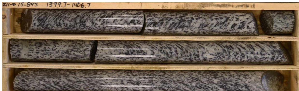
Figure 2-9: Typical FZ type (low-quartz) orthogneiss, with strong schistosity defined by obvious biotite-hornblende bands. The core box is 0.76 meters long.
