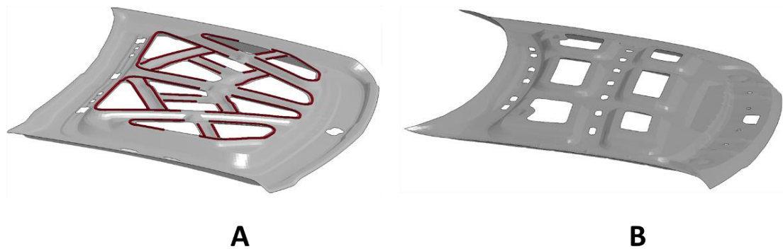
Figure 2-30 A) Inner hood structure with hood adhesive pads in pickup truck B) Inner hood structure in SUV
