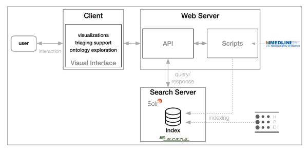
Figure 3-2 Client-server architecture of the OVERT-MED system. The webserver fetches MEDLINE updates from the NLM ftp site and indexes them in a Lucene index. HPO is also indexed. The API handles requests and connects to the Solr search server. The client displays visualizations and handles user interactions.
