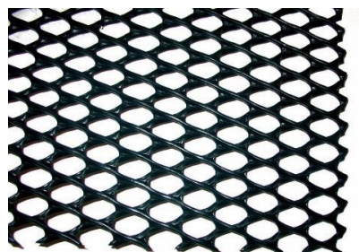
Figure 2-8: Geometric repetitive pattern of geonet material (source: Eith & Koerner, 1992)
