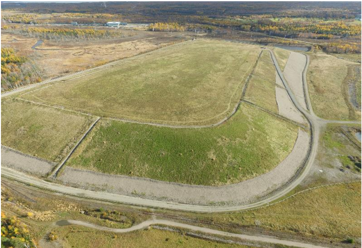
Figure 2-6: Distinct slope and plateau area of a waste rock pile in Sydney, Nova Scotia.
