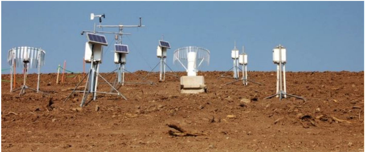
Figure 2-10: Monitoring equipment that can be used for cover performance evaluation (source: Ayres & O’Kane, 2013)
