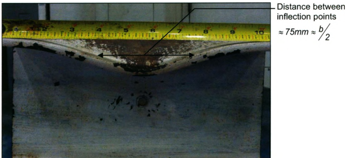
Figure 2-8: Local Buckle from a 4-Point Bending Test
