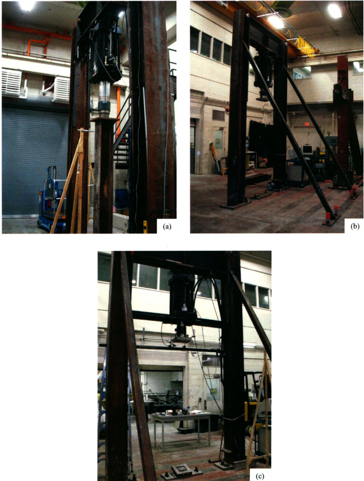
Figure 3-7: Implementation of Load Frame Bracing
