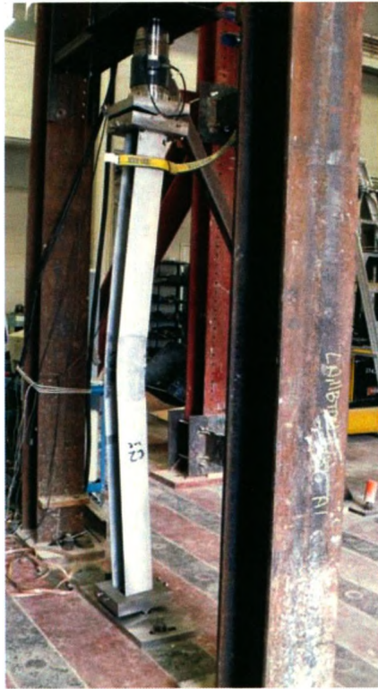
Figure 3-16: Plastic Hinge at Midheight (Column 2)
