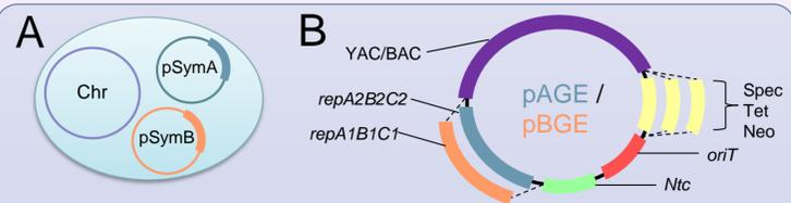
**Figure 1. Derivation of multi-host (MHS) shuttle vectors for Rhizobia.** **A)** The tripartite *S. melliloti* genome composed of a chromosome (Chr) and two megaplasmids (pSymA, pSymB). **B)** Components of MHS vectors derived from *S. melliloti* repABC origins, a Yeast and Bacteria Artificial Chromosome (YAC/BAC) backbone, an origin of transfer (*oriT*), a diatom selectable marker (*Ntc*), and Rhizobia selection markers (Spec, Tet, or Neo).
