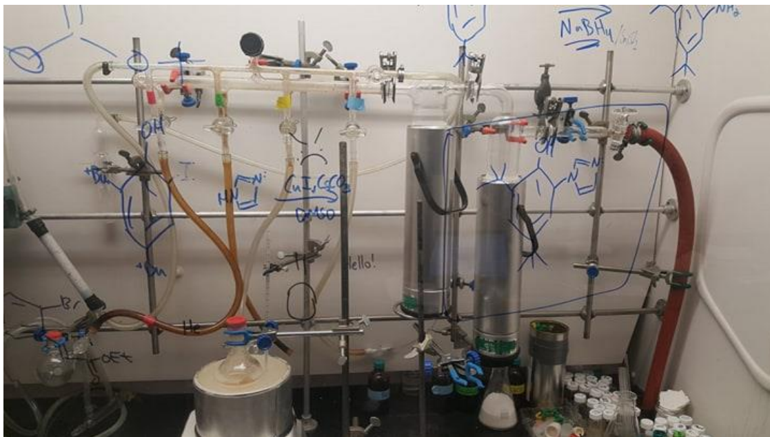
Appendix 1: Schlenk line setup for the first reaction.
