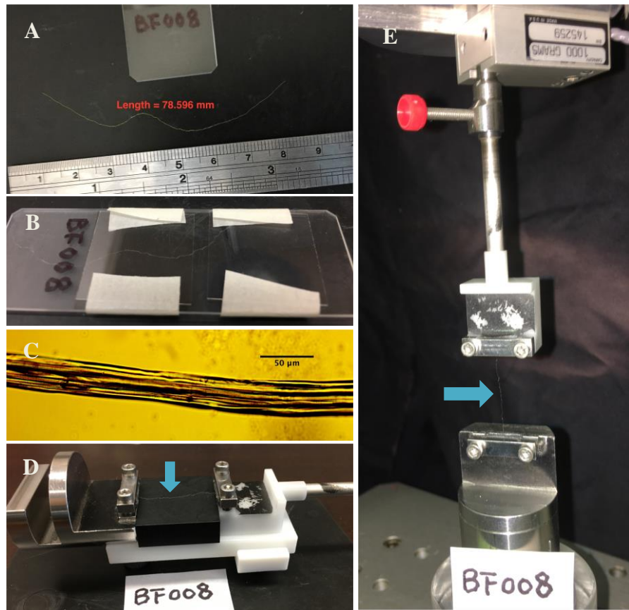
Figure 4-2: Property measurement process of a bamboo fiber
