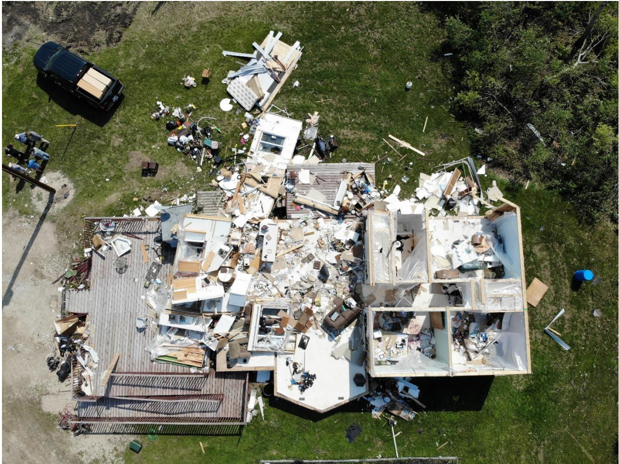
Figure 1: Aerial View of house that lost its roof in the Aug. 2018 Alonsa, MB tornado. I was one of two Western researchers sent to survey the damage.
