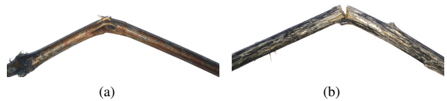
Fig. 7. (a) Buckling instead of breaking into pieces. (b) Greenstick fracture rather than breaking.
