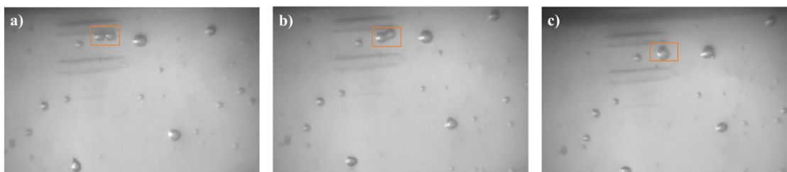
Figure 4.10: Images of bubble coalesce process in non-cavitation regime
