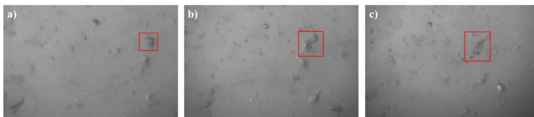
Figure 4.9: Images of bubble breakup in cavitation regime
