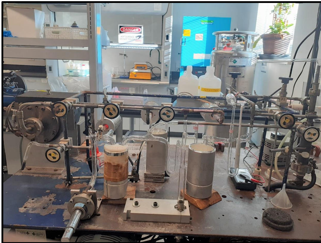
Figure 2-3 Photograph of argon extraction line showing the placement of the liquid nitrogen, used to trap condensable gases, and the MS 10 mass spectrometer (left).
