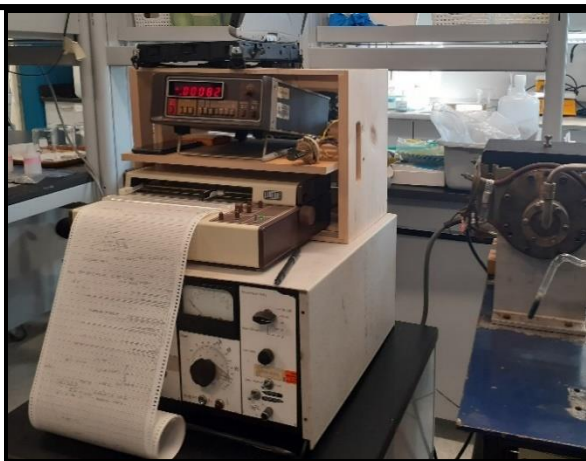
MS-10 Mass spectrometer controller
