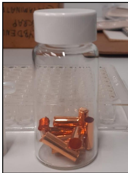
Copper capsules used to contain powdered clay fraction.
