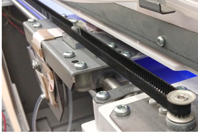
Figure 1: Belt and pulley configuration of x-y gantry 9
